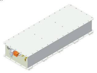
High-voltage lithium-ion battery based on highly efficient NMC cell technology, providing high power and durability. Its low weight and high energy density allow for the use of the battery to power buses and heavy-duty vehicles. The battery is equipped with a BMS (Battery Management System) that enables maintenance-free operation and allows for monitoring battery parameters through the CAN bus and service application.
