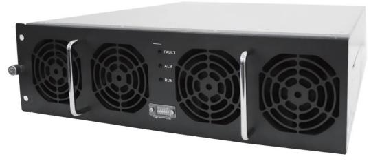
The module has been specially designed for DC electric vehicle chargers. It is characterized by its high efficiency, high power factor, high power density, and exceptional reliability. It features a 3-phase 4-wire AC input and offers a DC output voltage range from 150 to 1000VDC with an output power of 20kW. It is compliant with safety standards such as CE EN61851-1, EN61851-23 requirements, and EMC standard EN61851-21-2.
