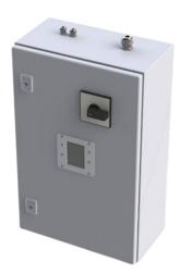
The device was designed to charge batteries and power power-electronics devices. It is characterised by high efficiency, high power factor, high power density and high reliability. It contains 3-phase 4-wire AC input, DC voltage output range is from 150 to 750VDC with an output power of 15kW, compliant with CE EN61851-1 safety regulation, EN61851-23 requirements and EN61851-21-2 EMC regulation.
