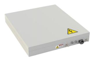
High voltage lithium-ion battery based on highly efficient NMC cell technology, providing high power and durability. Low mass and high density of the energy allows to use the battery to power buses and truck vehicles. The battery is equipped with BMS (Battery Management System), that enables maintenance-free operation and allows for monitoring battery parameters through the CAN bus and service application.
