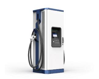
The EN120K2 charging station is used for fast charging electric vehicles. The product features high efficiency, power and reliability, as well as harsh environment resistance. It complies with global electric vehicle charging standards. The maximum DC charging power is 120kW. However, 150kW or 180kW configurations are possible. The maximum charging current reaches 300A. The unit is three-phase powered, with an available output voltage range of 150V to 1000V.
